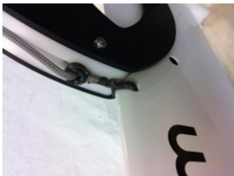
Assembly of the lowering line using a low friction ring
